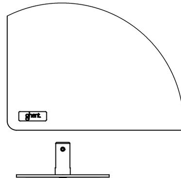
**Step 4:** Attach the feet to the acrylic panel by tightening the screw on the front of the bracket, wrench provided.
