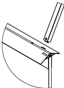
**Step 3:** Use the included wrench to tighten the socket screw. The screw must be completely tightened for a secure leg connection.
