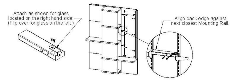
Step 14: Install Glass by carefully hooking onto the Glass Clamps. (If applicable)
