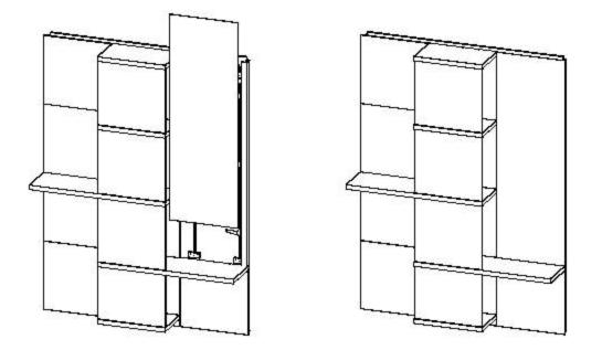
Step 15: Tighten top screws to secure structure. This is needed on all locations except for glass.
