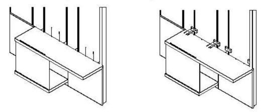
Step 10: Continue installing panels, shelving, polycarbonate and appropriate hardware as necessary.
