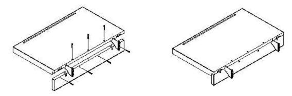
Step 6: Attach bottom shelf and stops. Screw in left and right holes for the stops first before the center.
