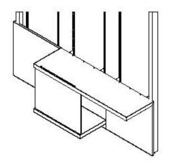
**Step 9:** Insert screws to connect the shelf to the vertical panels underneath. Ensure panels are fully straightened before fastening. Then mount Shelf Stop.
