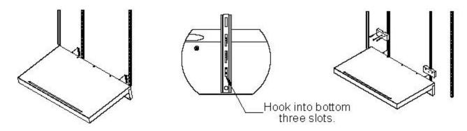
**Step 7:** Attach bottom panels. Ensure that the hooks are attached to the proper slots so that the bottom of the panel is about 1/8" below the rail.
