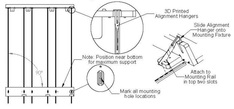
**Optional (Step 4):** If the Mounting Rails are not positioned directly in front of wooden studs then install anchors as needed.
