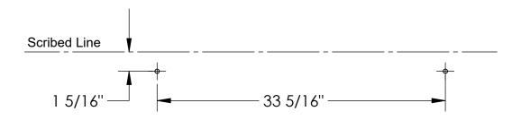
**Step 3:** Drill (2) marked holes. Use wall inserts to hold mounting screws. Carefully hang the board assembly on (2) screws.
