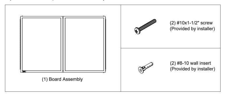
**Step 2:** Determine the desired mounting height of the VisuALL PC and scribe a level line 1-5/16" down from this location. Position and mark the locations for (2) mounting holes 33-5/16" apart.
